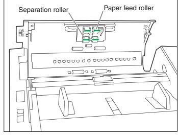
4 Open the double feed prevention conveyor in the direction of the arrow shown in the figure by using the indent on the back side.
